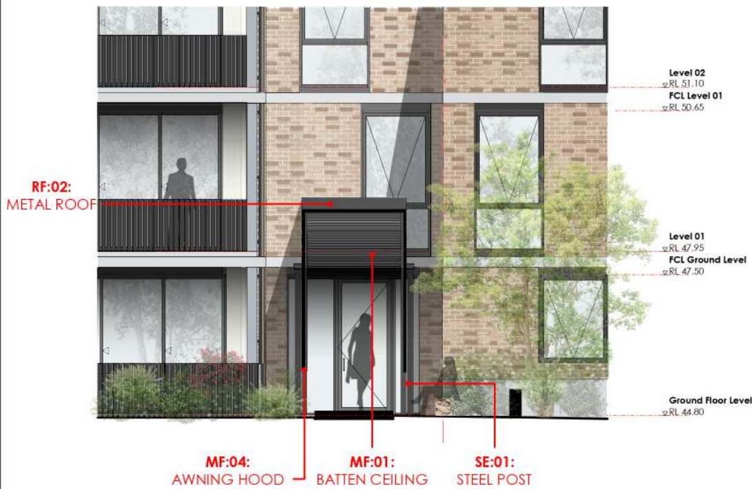
3 West Elevation - Entry Detail 1 : 50
